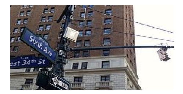
RFID E-ZPass reader attached to the pole and its antenna (right) used in traffic monitoring in New York City by using vehicle re-identification method
